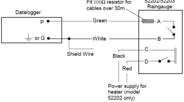
Figure 2 Wiring Diagram for 52202/52203
