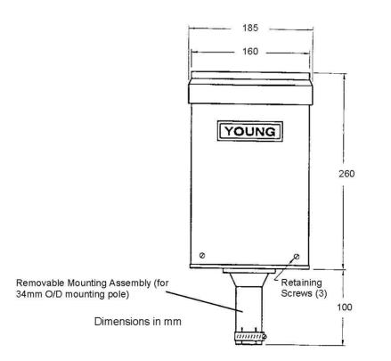
Figure 1 Dimensions of 52202/52203 Tipping Bucket Raingauge
